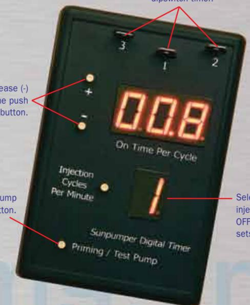
Select between multiple injection cycles(1-9). OFF Time sets automatically.
